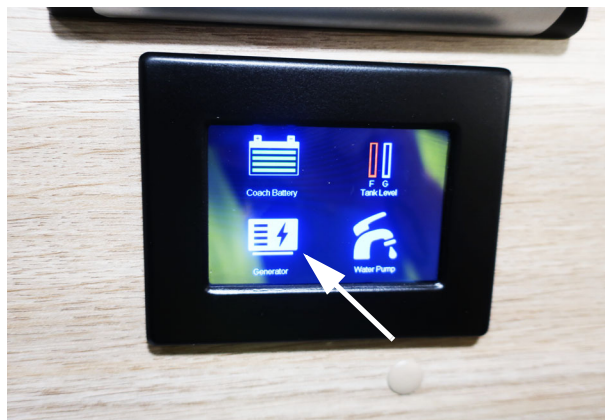
Generator location on the main screen of the Systems Monitor Panel -Typical View
