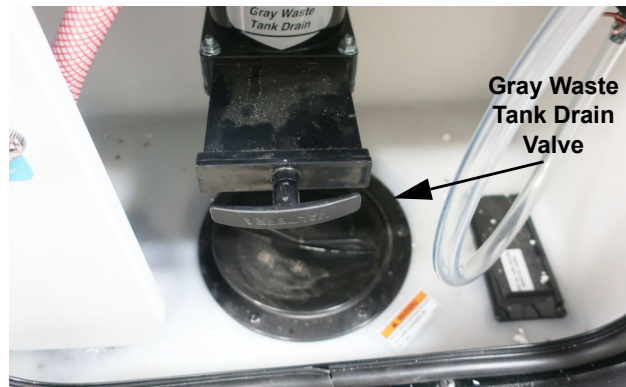
Sewage Drain outlet (Located inside the Water Service Center on the drivers side) -Typical View
