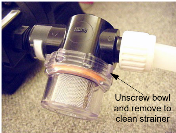
Water Pump Strainer -Typical View
