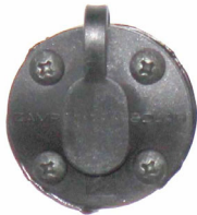
Single Solar Port (Located on the driver's side exterior of motorhome). -Typical View
