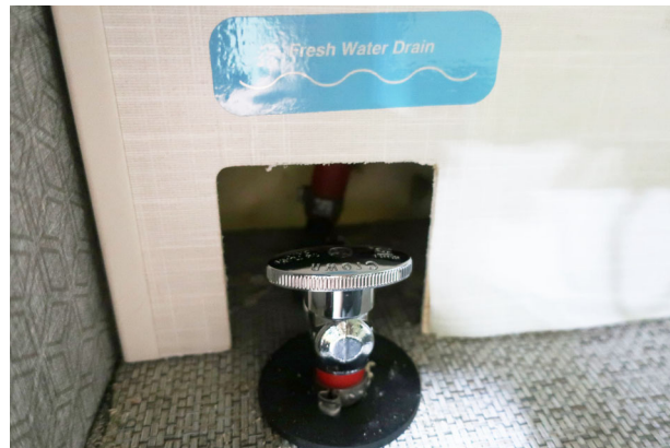
1 of the General Drain valves- the Tailgate Drain Valve. (Shown in the closed position) -Typical View
