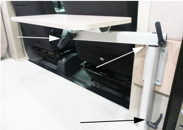
There are 3 adjustment levers that alter the height, length, and position of the table. -Typical View
