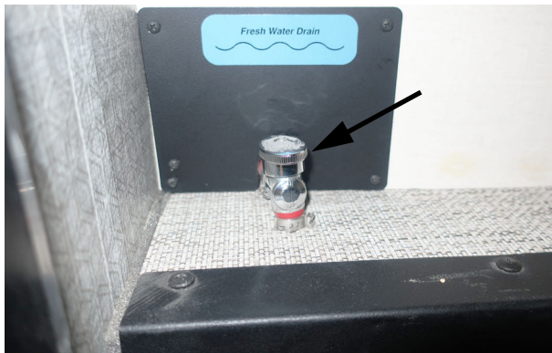
Open and drain the one General Waterline Drain- Passenger Compartment Drain Valve (Shown in the open position). -Typical View
