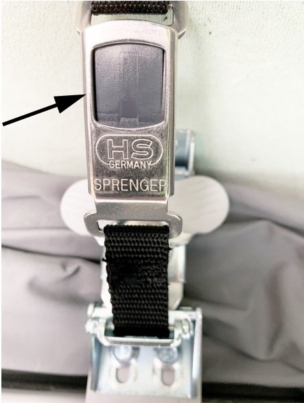
Locate the retention clamps on the driver's and passenger's side of the Pop-Top, and push the black button to release. -Typical View
